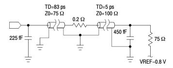
Figure 7: Receiver load model
