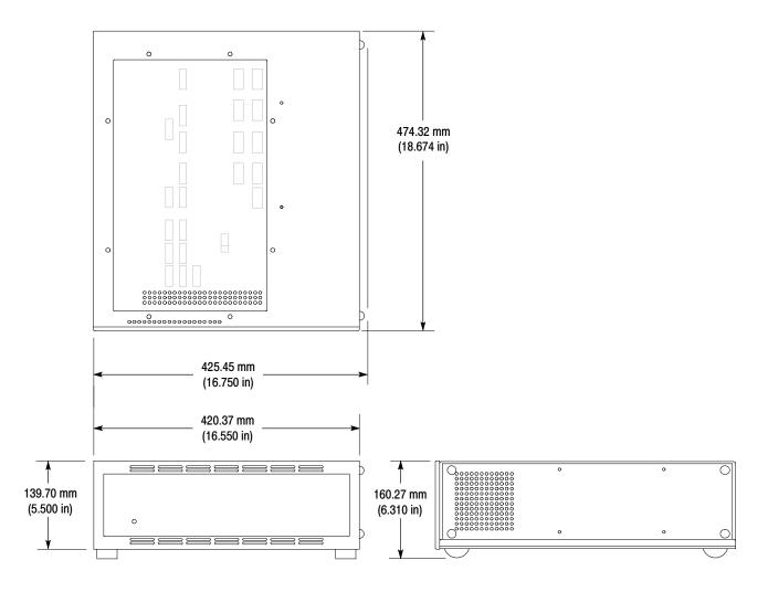
Figure 10: Dimensions of the preprocessor unit
