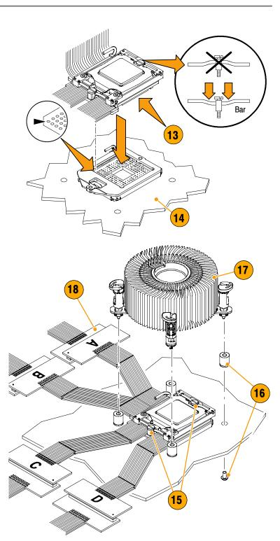
**LGA771 heat sink.** follow these steps to attach the TMSDPH2 probe head and the LGA771 heat sink kit hardware:
