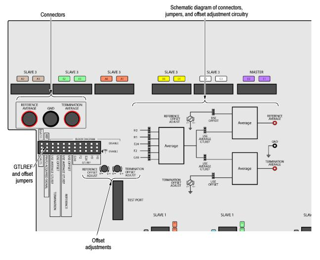
Figure 1: Preprocessor jumper, adjustment, and connector locations
