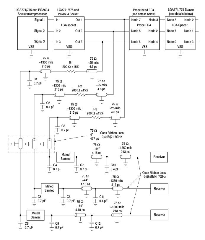
Figure 8: Electrical load model for typical signals
