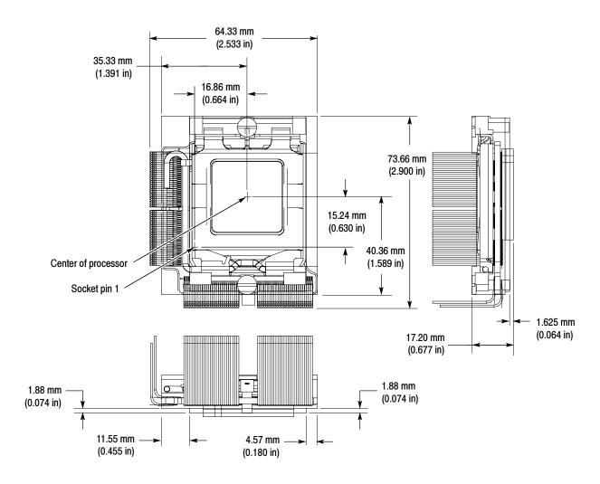
Figure 9: Dimensions of the probe head
